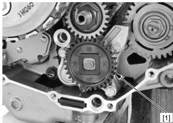
Remove the oil pump mounting bolts [1] and oil pump assembly bolt [2].
