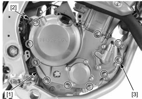
Connect the water hose [1] and tighten the water hose band screw [2] (page 9-7).
