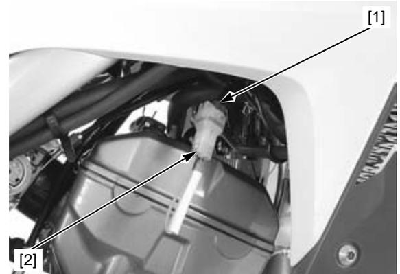
5. Disconnect the ECT sensor 3P connector [1].
