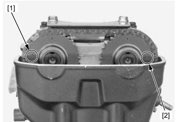
Check the valve clearance by inserting a feeler gauge [1] between the rocker arm and shim.
