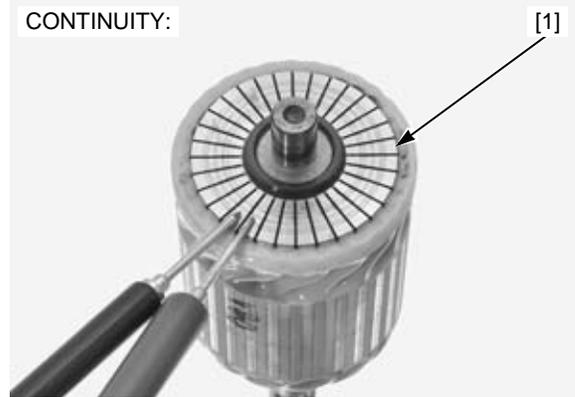
Check for continuity between each individual commutator bar [1] and the armature shaft [2].
