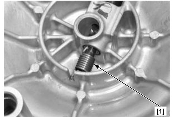
Remove the clutch lifter arm [1] from the right crankcase cover.
