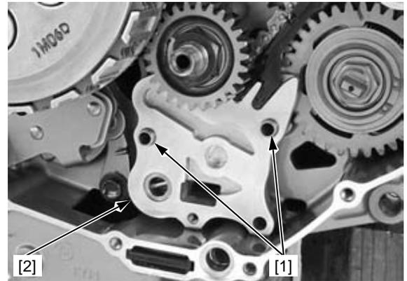
Remove the oil pump body [1] by releasing it from the cam chain guide hook [2] and pressure relief valve [3].
