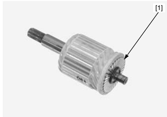
Check for continuity between pair of commutator bars [1].
