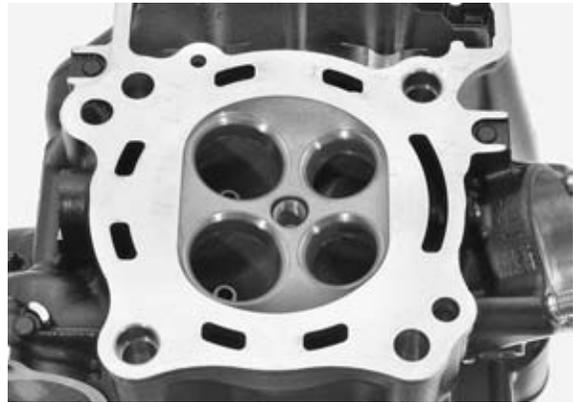
Support the cylinder head and drive out the valve guides from the combustion chamber side of the cylinder head.
