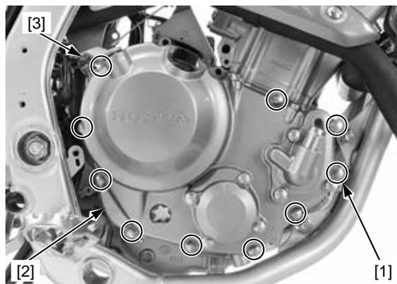
Remove the dowel pin A [1], dowel pin B [2] and gasket [3].
