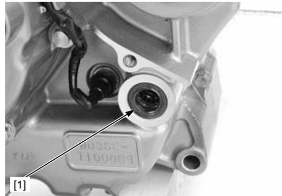
*Be careful not to let the removed parts fall into the crankcase.* Remove the shift drum stopper plate bolt [1].
